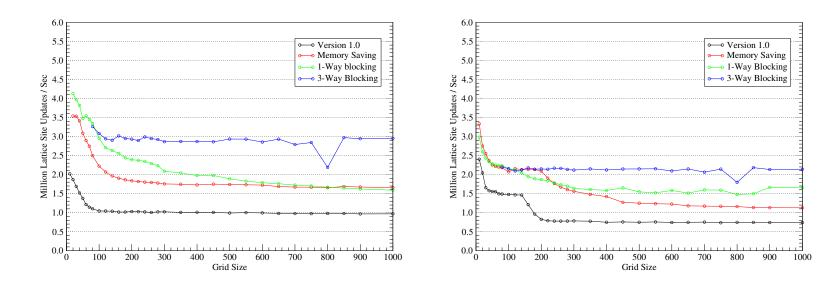
left: 2D LB code, AMD Athlon machine, 700 MHz right: 2D LB code, Alpha A21164 machine, 500 MHz
