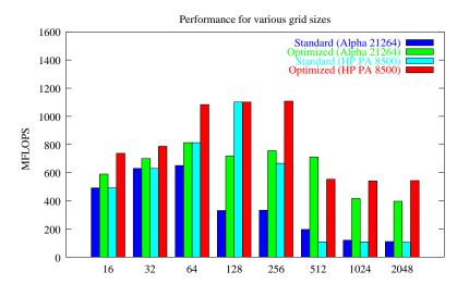
Variable–coefficient problems: speedup factors of 2–3 can be obtained for large grids, the MFLOPS rates are usually smaller since much more data have to be loaded
