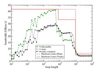
Fig. 2. Serial vector bandwidth triadItanium2 using different memory allocation strategies. The bandwidth limits imposed by the hardware are depicted as well, Plain denoting the pure hardware numbers and Triadstaking into account the additional load operation if an L2/L3 write miss occurs.
