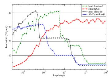
Fig. 1. Memory bandwidth vs. loop length N for the serial vector triad on several architectures.
