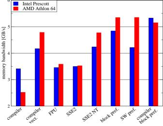
Fig. 4. Serial vector triad main memory bandwidth on Intel Prescott and AMD Athlon64
