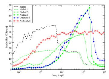
Fig. 6. Memory bandwidth vs. loop length N for the shared-memory parallel triad on SGI Altix (Itanium2) and one SX6+processor.
