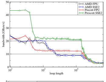
Fig. 3. Serial vector triad bandwidth on Intel Prescott and AMD Athlon64: comparison of SSE2 and FPU versions.
