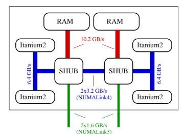
Fig. 5. SGI3700 Altix  $\operatorname{SC-brick}$ block diagram. One SC-brick comprises two nodes with two CPUs each. Intra-brick communication is twice as fast as brick-to-brick communication
