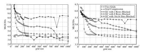
Figure 7: Performance in millions of lattice site updates per second (MLSUD/s) on machines based on an AMD Athlon XP 2400+ (left) and on an Intel Itanium2 (right), respectively, for various grid sizes.
