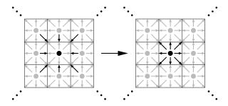
Figure 2: Representation of the LBM updating a single lattice site by a stream operation (left) and a subsequent collide operation (right).
