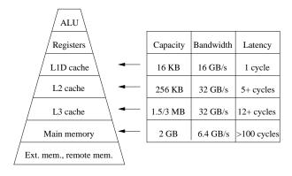
Figure 1: Memory architecture of a workstation based on an Intel Itanium 2 CPU with three levels of on–chip cache [12].
