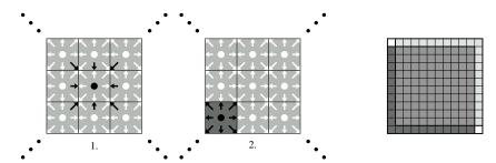
Figure 4: Fused stream—and—collide step for the cell in the middle (left, 1 and 2), layout of the two overlayed grids after applying the grid compression technique (right).
