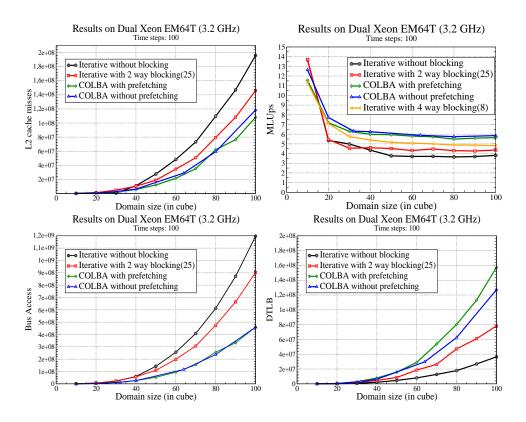
Figure 2: Comparison between COLBA and iterative algorithm for the D3Q19 model. a) Cache misses (top left) b) Mega Lattice site Updates per second. (MLUps) (top right) c) Buss access (bottom left) d) DTLB misses (bottom right).
